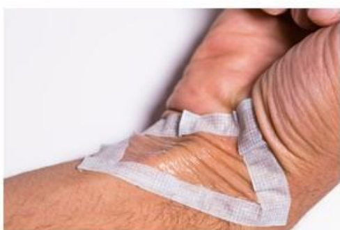
Fig. S20. Prevention of delamination during extreme deformation via adhesive design. Optical images of silicone adhesive, with E \sim 100 kPa and q_{\text{adhesion}} = 160 N/m with tape frame, on the wrist of a human subject illustrating conformal contact during extreme deformation.
